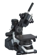
Free-angle observation system VH-S300 (manual)
