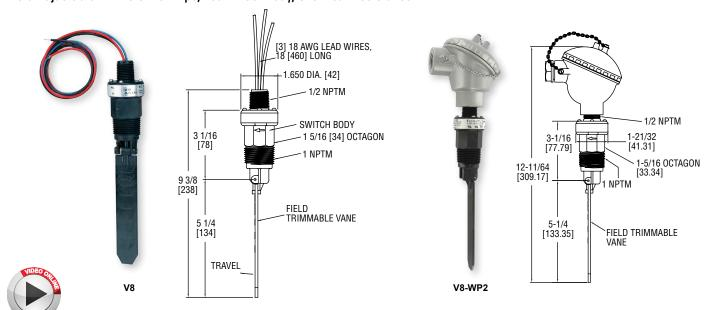
The SERIES V8 Flotect® Vane Operated Flow Switches is ideal for protecting unattended equipment from damage or loss of production. This Series is available for installation in a 1 to 6" pipe with operating pressures are up to 150 psig (10 bar) and temperatures to 212°F (100°C).
