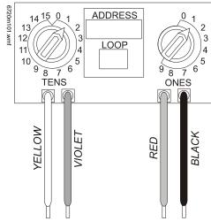
The TC809B Mini Monitor Module can be installed in a singlegang junction directly behind the monitored unit. Its small size and light weight allow it to be installed without rigid mounting. The TC809B is intended for use in intelligent, two-wire systems where the individual address of each module is selected using rotary switches. It provides a two-wire initiating device circuit for normally-open-contact fire alarm and security devices.
