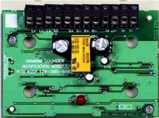
Fig. 1: SNM800 Sounder Notification Module
