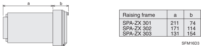
Fig. 3 Semi-flush mounting relay case (dimensions in mm)
