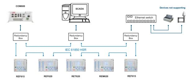
The choice between the HSR and PRP redundancy protocols depends on the required functionality, cost and complexity.
