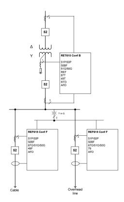
Figure 3. Illustrates the protection of a two winding power transformer with configuration B. The main protection used in this application example is transformer differential protection. Additionally, restricted ground fault protection with numerical low impedance principal is applied on the transformer's LV side.
