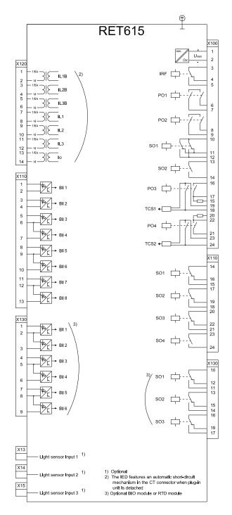
Figure 15. Terminal diagram of standard configuration F
