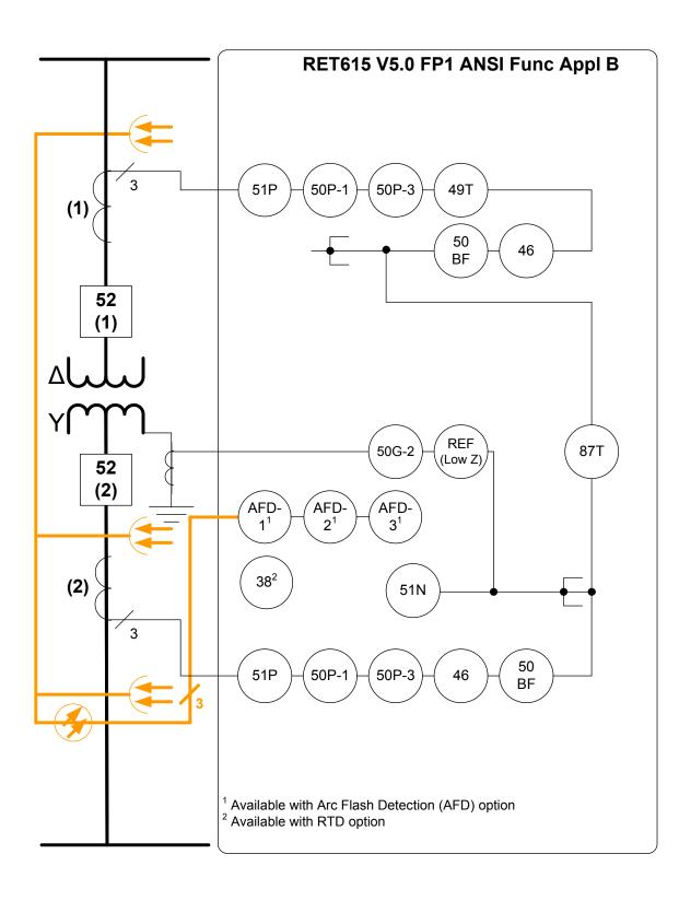
Figure 2. Functionality overview for standard configuration F
