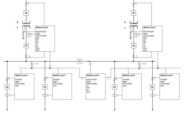
Figure 4 Illustrates the protection of the two winding power transformers feeding a double ended substation. In this case configuration F provides the main protection for the transformers: differential protection and low impedance restricted ground fault protection. In addition configuration F provides the main protection for the incoming feeders also, and it includes synchcheck control and directional overcurrent protection in case incoming feeders will be momentarily paralleled.
