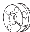
Type 2.6 Clamping hub double slot, with feather keyway Positive locking power transmission with additional frictionally engaged condition. The frictionally engaged condition prevents or reduces reverse backlash, respectively. Surface pressure of the keyway connection is reduced.
