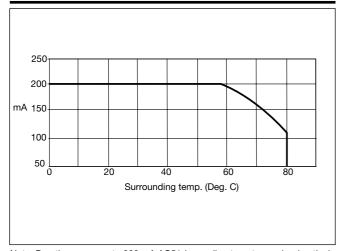
Note: Derating curve up to 200 mA AC51 (according to optocoupler derating)
