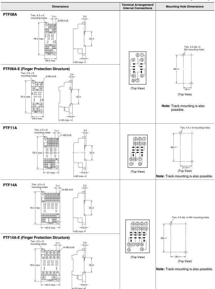
Note: If you use the PTF08A, PTF08A-E, or PT08 with an LY1 Relay, connect the following terminal pairs: 1-2, 3-4, and 5-6 (for usage at 10 A or higher).
