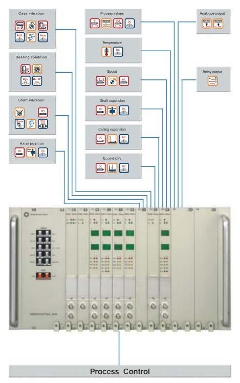
VIBROCONTROL 4000 allows continuous monitoring of all measurement variables that are monitored today for assessment of machine condition:
