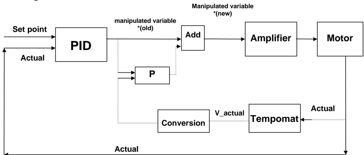
The PID controller in the FOX-20 is a PID controller with variable structure. The mathematical description is given below.
