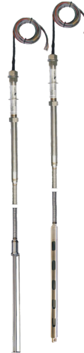
WLS integrated with MST sensor (MSTW), open model to the left and closed model to the right. It is hung vertically from the top of the tank, and the position/length is chosen according to the actual bottom water range. The WLS should be anchored to the tank bottom to ensure a fixed position in case of turbulence.
