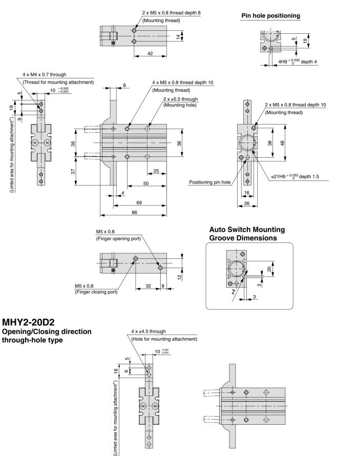
\* Do not extend the attachment from limited area for mounting to avoid interference with the attachment or main body.
