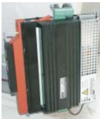
Figure 14: Size 0 with installed braking resistor BW090-P52B
