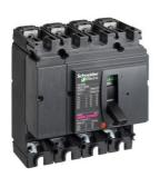
Circuit breaker basic frame, ComPact NSX250H, 70kA at 415VAC 50/60 Hz, 250A, without trip unit, 4 poles
