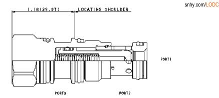
These unbalanced, pilot-to-close logic valves are 2-way switching elements that are spring biased closed. Pressure at either work port 1 or 2 will oppose the spring and tend to open the valve while pressure at port 3 will tend to close it. The force generated at port 3, plus the spring force, must be greater than the sum of the forces acting at port 1 and port 2 for the valve to remain closed. NOTE: The pilot area (port 3) is 1.8 times the area at port 1 and 2.25 times the area at port 2.
