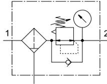
Condensate drain, fully automatic, with pressure gauge
