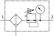
Condensate drain, semi- or fully automatic, with pressure gauge
