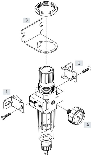
Individual unit without connecting plates, for service unit combination
