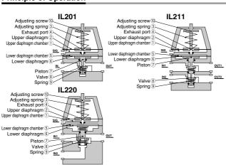
The signal air pressure enters the upper diaphragm chamber ① to generate a force. When this force is larger than the force generated by compressing the adjusting spring ③, the upper diaphragm ② is pushed up, the exhaust port ④ is closed, and the signal air pressure enters the lower diaphragm chamber ⑤ and acts the lower diaphragm ⑥. This pushes down the piston ⑦ to open the valve.
