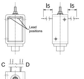
Fig. 4: Type G FC X... flying lead placement
