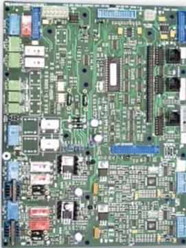
The Field Interface Module FIM is the main interface for field wiring on MX detection panels and contains plug-in field wiring terminals, inter board connectors, EMC protectors and filters and general I/O electronics. The FIM801 and FIM801CV provides 1 x MZX DIGITAL loop and the FIM802 provides 2 x MZX DIGITAL loops. Each MZX DIGITAL loop can support several kilometres of loop wiring using a mixed topology using multiple loops and spurs.
