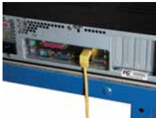
Down cable: cable clip faces down and the cable angles down. Shown: EVNSL24E-0003-90DS
