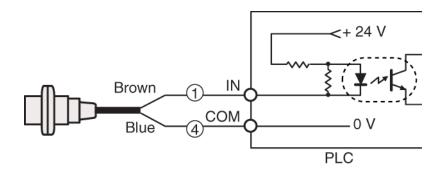
Connection to PLC having no internal DC power supply
