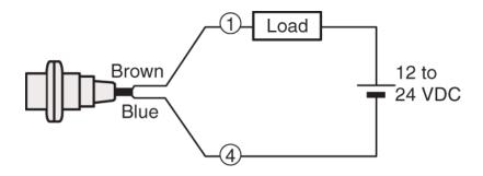
Connection to built-in DC power supply type PLC (internally connected power supply
