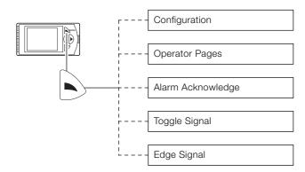
Fig. 6: Programmable soft key
