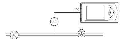
Fig. 12: Single PV with totalization
