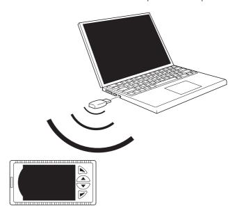
Fig. 10: Transferring a configuration file via the infrared port
