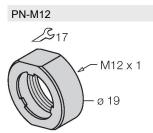
6905309 Impact protection nut for M12x1 threaded barrel devices; material: Stainless steel A2 1.4305 (AISI 303)
