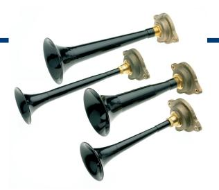
The SK Series of air horns are manufactured from non-ferrous materials which offer high corrosion and weatherproof resistance for use in railway and marine applications as well as general purpose signalling. Operated from a compressed air supply, their powerful high output low frequency sound cuts through background noise to provide an effective warning. Optional compressor available for applications which do not have an on-site air supply.
