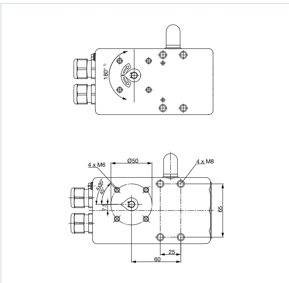
1.) For the EtherNet/IP, PROFINET, Modbus TCP and büS versions a max. of  $180^\circ$  is possible, for the other versions max.  $150^\circ$ .
