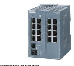
SCALANCE XB216 managed layer 2 IE switch, 16X 10/100 Mbit/s RJ45 ports, 1x console port, diagnostics LED red redundant power supply; IEC 62443-4-2 certified; temperature range 0 to +60 °C DIN-rail mounting; default EtherNet/IP.
