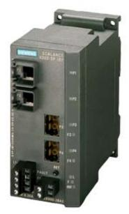
SCALANCE X202-2PIRT managed IE IRT switch, 2x 10/100 Mbit/s RJ45 ports, 2x 100 Mbit/s POF SC RJ ports, Error signaling contact with set button, Redundant power supply, PROFINET IO device, network management, Redundancy Manager integrated, incl. electron. manual on CD-ROM, C-plug optional
