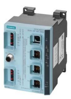
SCALANCE X201-3PIRT PRO; managed IE IRT Switch Degree of protection IP65/67; 1x 10/100 Mbit/s Push Pull RJ45 port; 3x 100 Mbit/s Push-pull SCRJ port; Error signaling contact with set pushbutton; Redundant power Supply; PROFINET IO device; network management; Redundancy Manager integrated, incl. electron. manual on CD-ROM, C-plug optional
