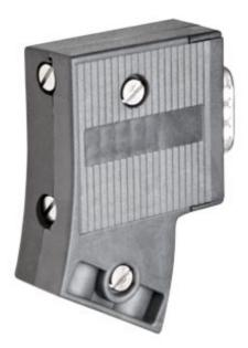
SIMATIC DP, bus connection plug f. PROFIBUS w. inclined cable outlet, max. 1.5 Mbaud, insulation displacement method, 15x 57.6x 39.5 mm (WxHxD), without bus terminating resistor and programming device socket
