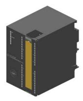
SIMATIC S7, Digital input SM 326, 8 DI; 24 V DC, NAMUR, fail-safe NAMUR input for SIMATIC S7 F-systems, up to Category 4 (EN 954-1)/ SIL3 (IEC61508)/PLE (ISO13849), 1x 40-pole
