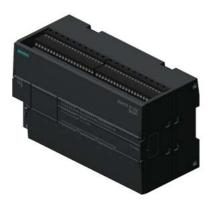
\*\*\* spare part \*\*\* SIMATIC S7-200 SMART, CPU SR60, CPU, AC/DC/relay, onboard I/O: 36 DI 24 V DC; 24 DO relay 2 A; power supply: AC 85-264 V AC at 47-63 Hz, program/data memory 50 KB
