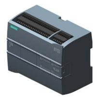
SIMATIC S7-1200, CPU 1215C, compact CPU, DC/DC/DC, 2 PROFINET ports, onboard I/O: 14 DI 24 V DC; 10 DO 24 V DC; 0.5A; 2 AI 0-10 V DC, 2 AO 0-20 mA DC, Power supply: DC 20.4-28.8V DC, Program/data memory 125 KB
