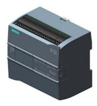
SIMATIC S7-1200, CPU 1214C, compact CPU, DC/DC/relay, onboard I/O: 14 DI 24 V DC; 10 DO relay 2 A; 2 AI 0-10 V DC, Power supply: DC 20.4-28.8V DC, Program/data memory 100 KB
