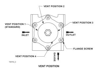
Figure 4. 67C Series Vent and Drain Valve Positions
