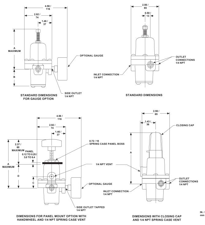
Figure 5. Types 67C, 67CR, 67CS and 67CSR Dimensions
