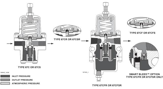
Figure 2. 67C Series Operational Schematics
