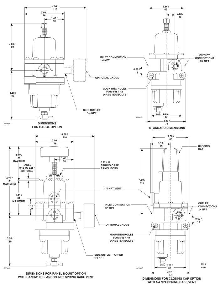
Figure 6. Types 67CF and 67CFR Dimensions
