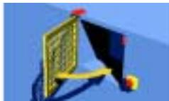
**Note:** Lift-off guards require good alignment when using tongue actuated interlock switches.
