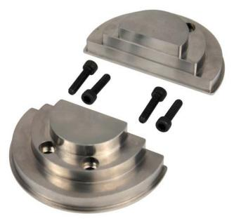
The stepped cable tie bollards are symmetrical allowing for easy use and fitment. The stepped design allows the fixture to test an array of common cable tie sizes. Two M5 cap-head bolts secure each section of the fixture.
