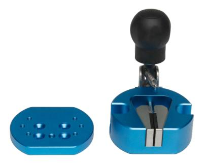
The quick release spring action allows easy loading and unloading of samples. Two M5 cap-head bolts secure the wedge-action terminal grip mounting plate to the tester. Suitable for wire with a diameter up to 8mm.
