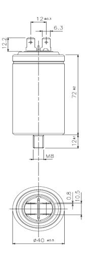
Total elongation is about 10 mm after the overpressure disconnector release. Don't use rigid connections.
