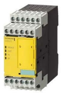
!!! Phased-out product !!! The successor product series is 3SK2 (see FAQ 109741483) SIRIUS safety relay with relay enabling circuits (EC) 24...240 V UC, 45 mm overall width screw terminal EC instantaneous: 2 NO EC delayed: 2 SC: 3 Switch with 8 functions Basic device Maximum achievable PL according to EN 13849-1: Maximum achievable SIL according to IEC 61508: 3
