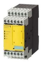
!!! Phased-out product !!! The successor product series is 3SK2 (see FAQ 109741483) SIRIUS safety relay with relay enabling circuits (EC) 24...240 V UC, 45 mm overall width screw terminal EC instantaneous: 4 NO EC delayed: 0 SC: 2 Switch with 8 functions Basic device Maximum achievable PL according to EN 13849-1: Maximum achievable SIL according to IEC 61508: 3
