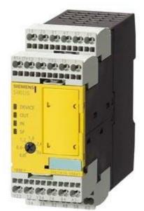
!!! Phased-out product !!! The successor product series is 3SK2 (see FAQ 109741483) SIRIUS safety relay with relay enabling circuits (EC) 24 V DC, 45 mm screw terminal EC instantaneous: 2 NO EC delayed: 2 SC: 4 Switch with 8 functions Basic device Maximum achievable PL according to EN 13849-1: Maximum achievable SIL according to IEC 61508: 3
