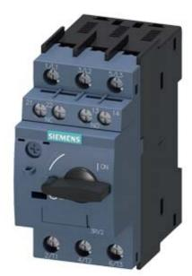
CIRCUIT-BREAKER SZ S00, FOR MOTOR PROTECTION, CLASS 10, A-REL. 2.2...3.2A, N-RELEASE42A, SCREW CONNECTION, STANDARD SW. CAPACITY W. TRANSVERSE AUX. SWITCH 1NO+1NC
