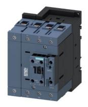
Power contactor, AC-3 65 A, 30 kW / 400 V 2 NO + 2 NC 20-33 V AC/DC 4-pole Size S3 screw terminals 1 NO + 1 NC integrated
