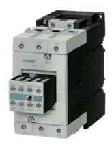
Power contactor, AC-3 80 A, 37 kW / 400 V 24 V DC, 2 NO + 2 NC 3-pole, Size S3 Screw terminal !!! Phased-out product !!! Successor is SIRIUS 3RT2 Preferred successor type is >>3RT2038-1KB44<<
