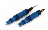
The Rosemount 3900 and 3900VP General Purpose pH/ORP Sensors feature a chemically resistant Ryton® plastic body, along with a built-in solution ground for advanced diagnostics and a Pt-100 resistance temperature device (RTD) for temperature compensation. These sensors are available with either an integral cable connection (Rosemount 3900) or Variopol (VP8) connector (Rosemount 3900VP). Variopol cables are sold separately (see Accessories).
