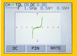
Huntron SigAssist is displayed at the top of the screen and is used to calculate and display numeric values based on the range parameters. The values displayed are resistance (in ohms), capacitance (in farads), power (in watts), and forward and reverse breakdown voltage (in volts).
