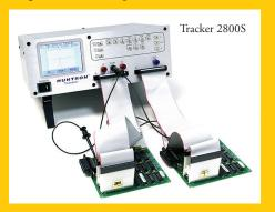
Comparisons between Channel A (green signature) and Channel B (red signature) can take place manually or automatically allowing you to identify signature differences quickly. The Tracker 2800S can save you time when compared to testing with hand probes. You can step through each pin using the touch screen controls, have the Tracker step through the pins at a preset rate or use the optional Huntron Workstation scan and compare for you.
