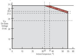
The area within the curve represents the safe operating range for the module under various conditions of user supplied 24V dc supply voltages and ambient temperatures.
