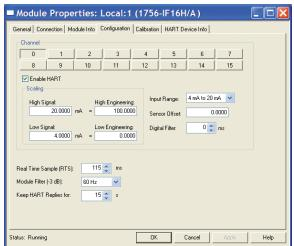
Each channel can be scaled with engineering units, filtering and real-time sample rate. Each channel is selectable for "current only" or "current and HART" for increased information availability. There is no need for application code to access the HART data. PV, SV, TV, FV and the associated status tags are in the module data structure.
